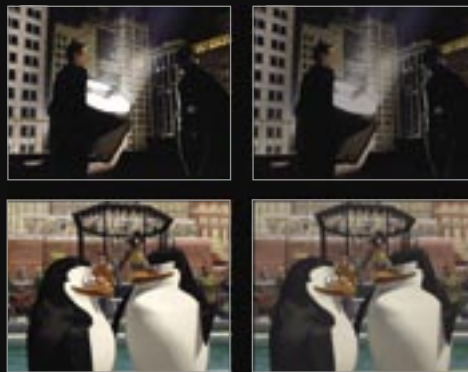
Top: Intensive white and deep black in the same picture with true optical contrast - deep black, but reduced whites with dynamic contrast.
